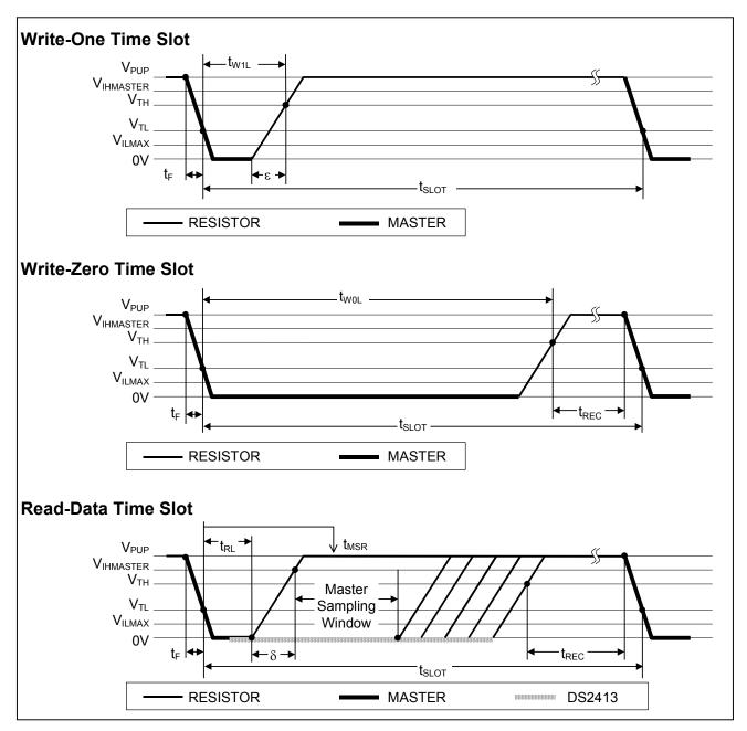
Figure 12. Read/Write Timing Diagram
