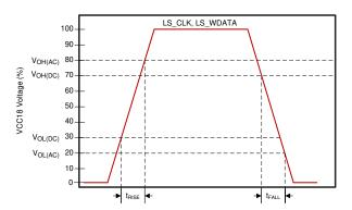
Figure 6-3. LS\_CLK and LS\_WDATA Slew Rate
