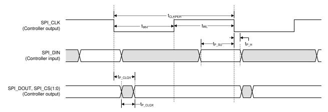
Figure 6-9. Flash Interface Timing
