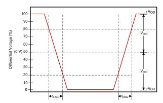
$V_{\text{CM}}$  is removed when the signals are viewed differentially.
