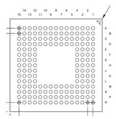
Figure 5-1. ZVB Package 176-Pin NFBGA Bottom View
