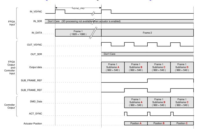
Figure 7-1. 2D Actuator Frame and Signal Timing
