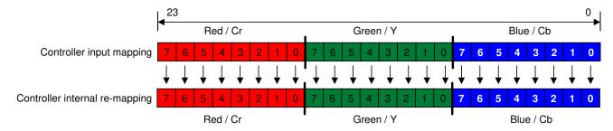
Figure 7-2. RGB-888 I/O Mapping
