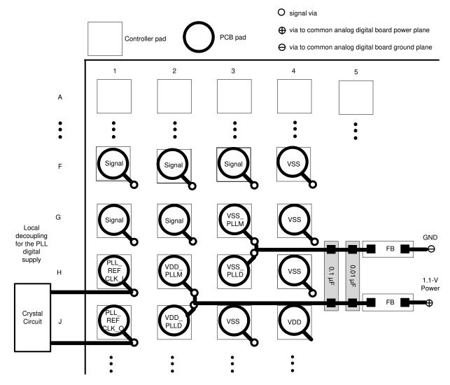
Figure 10-1. PLL Filter Layout
