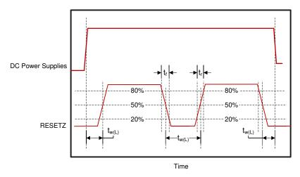
Figure 6-6. Power-Up and Power-Down RESETZ Timing
