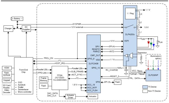
Figure 8-1. Typical Application Diagram (using DLPA200x)
