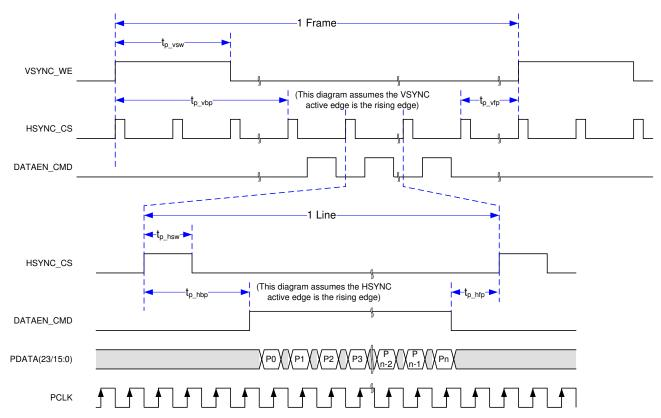
Figure 6-7. Parallel Interface Frame Timing
