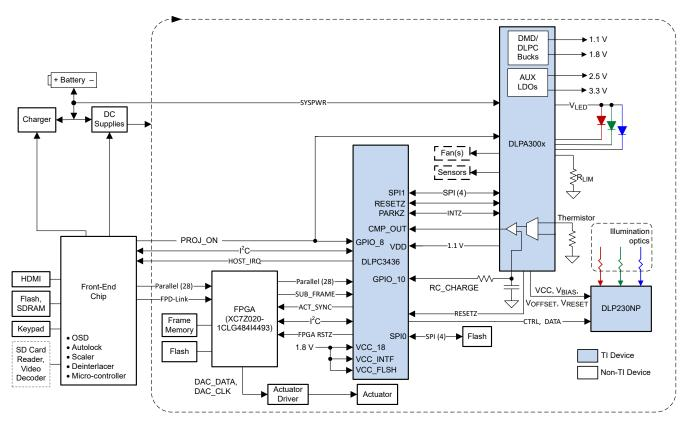
Figure 8-2. Typical Application Diagram (using DLPA300x)
