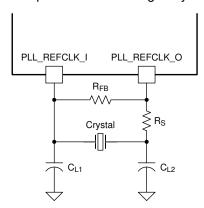
$$\begin{split} &C_L = \text{Crystal load capacitance (farads)} \\ &C_{L1} = 2 \times (C_L - \text{Cstray\_pll\_refclk\_i}) \\ &C_{L2} = 2 \times (C_L - \text{Cstray\_pll\_refclk\_o}) \\ &\text{where:} \end{split}$$
