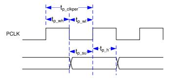
Figure 6-8. Parallel Interface Pixel Timing
