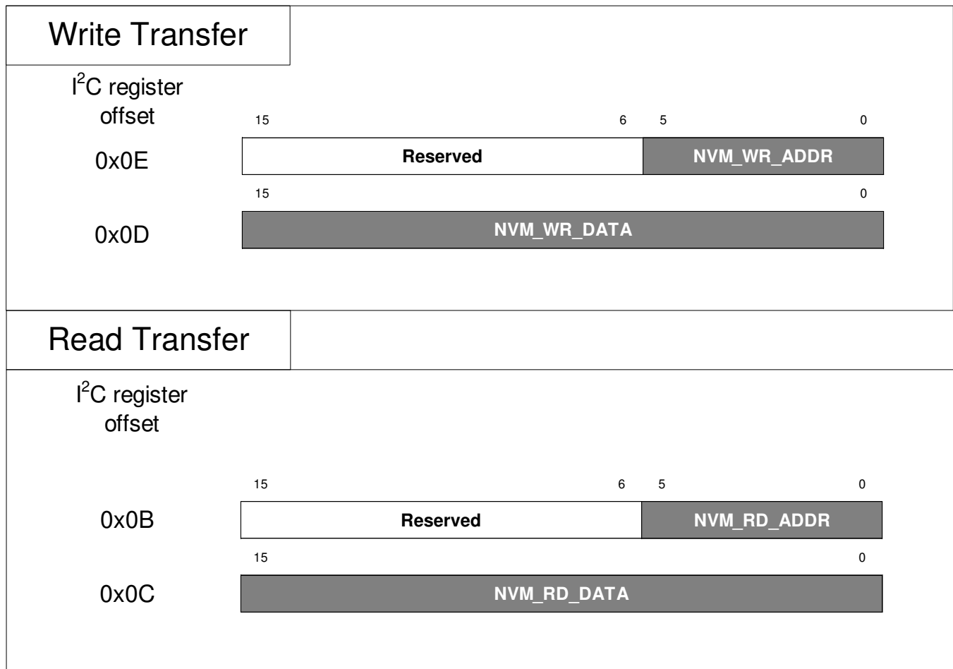
Figure 34. EEPROM Direct Access Using I 2 C
