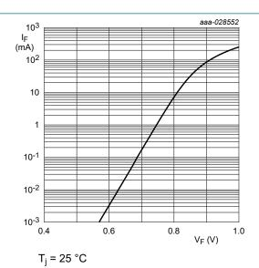
Fig. 4. Forward current as a function of forward voltage; typical values (BZB984-C7V5)
