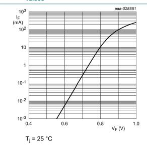
Fig. 3. Forward current as a function of forward voltage; typical values (BZB984-C6V8)
