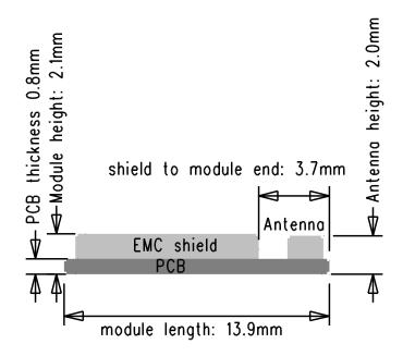
Figure 24 BT121 module side view dimensions
