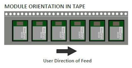
Figure 26 Module orientation in tape and feed direction
