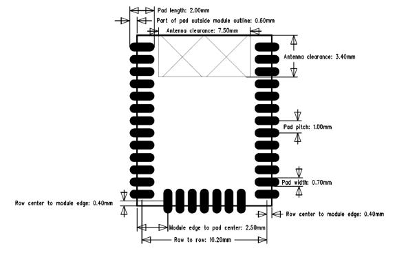
Figure 23 BT121 module recommended PCB pad pattern
