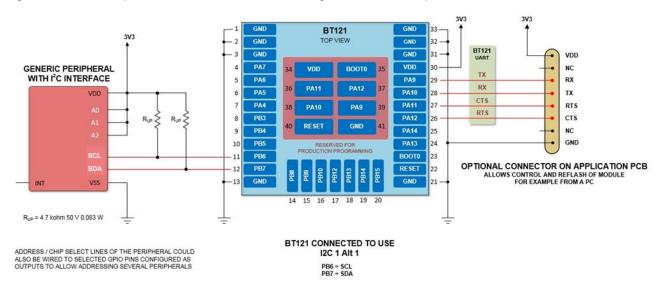
Figure 21 Connecting to an I2C peripheral
