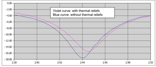
Figure 7 Typical antenna matching
