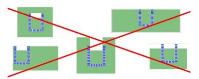
Figure 2 PCB layout recommendations for BT121 application boards
