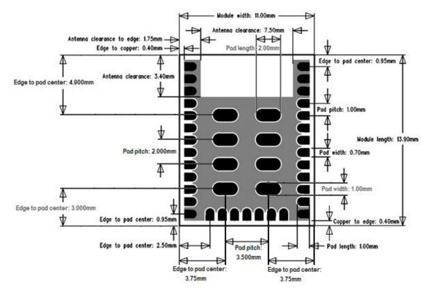
Figure 22 BT121 module physical dimensions
