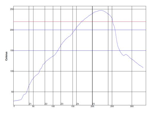
Figure 25 Reference reflow profile example
