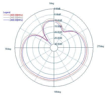
Figure 15 Typical 2D radiation pattern for BT121 with view from above module
