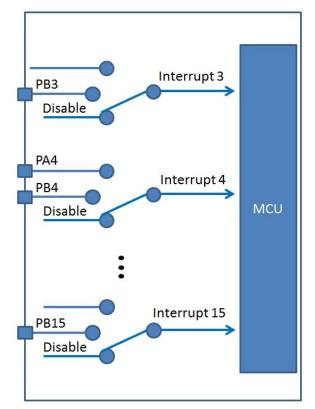
Figure 6 GPIO interrupt multiplexing scheme
