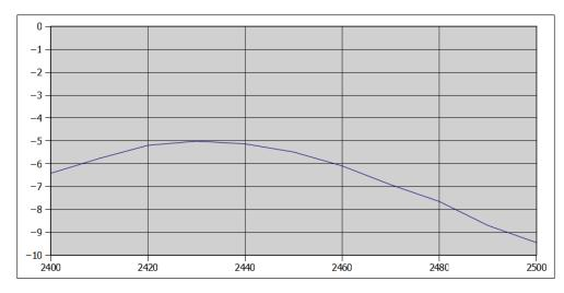
The measured antenna efficiency as a function of frequency is shown in *Figure 11* below.
