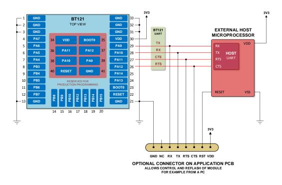
Figure 19 Connecting an external host with BT121 using UART
