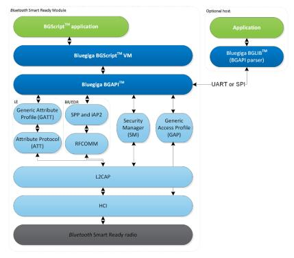
Figure 18 Bluegiga Bluetooth Smart Ready software stack
