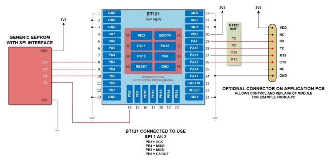
Figure 20 Connecting an external device with BT121 using SPI interface
