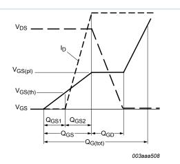
Fig. 15. MOSFET transistor: Gate charge waveform definitions
