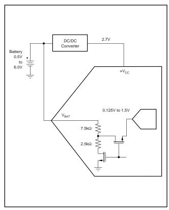
FIGURE 7. Battery Measurement Functional Block Diagram.
