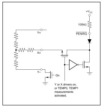
FIGURE 15. ADS7846 PENIRQ Functional Block Diagram.
