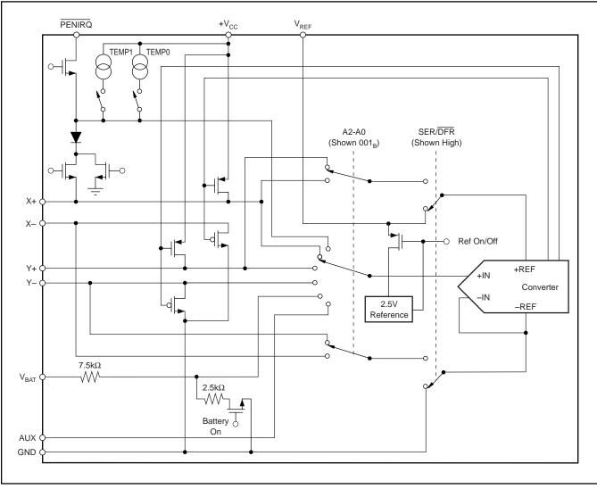
FIGURE 2. Simplified Diagram of Analog Input.
