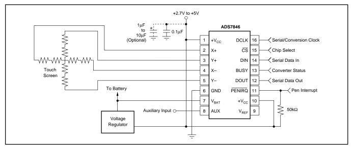
FIGURE 1. Basic Operation of the ADS7846.
