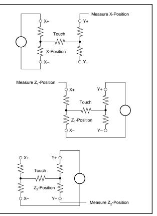
FIGURE 8. Pressure Measurement Block Diagrams.
