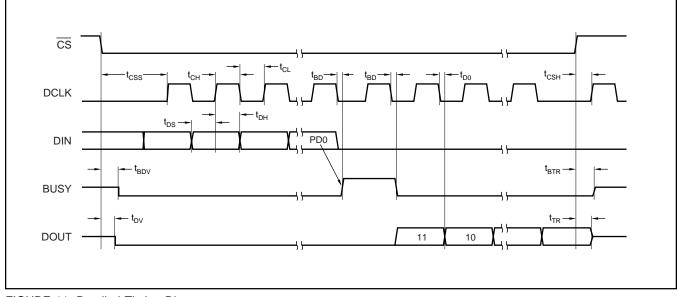
FIGURE 11. Detailed Timing Diagram.
