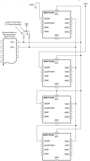
NOTE: The ADS111x-Q1 power and input connections are omitted for clarity. The ADDR pin selects the I<sup>2</sup>C address.
