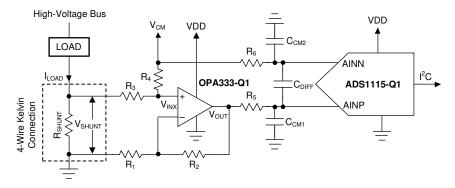
Figure 9-6. Low-Side Current Shunt Monitoring
