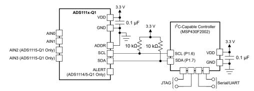
Figure 9-5. Basic Hardware Configuration
