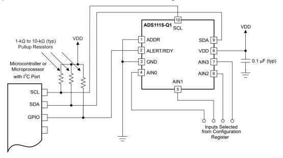
Figure 9-1. Typical Connections of the ADS1115-Q1
