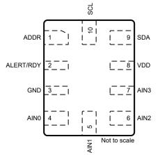
Figure 5-1. NKS Package, 10-Pin UQFN (Top View)
