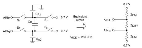
Figure 8-5. Simplified Analog Input Circuit
