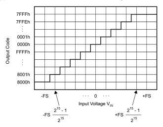
Figure 8-12. Code Transition Diagram
