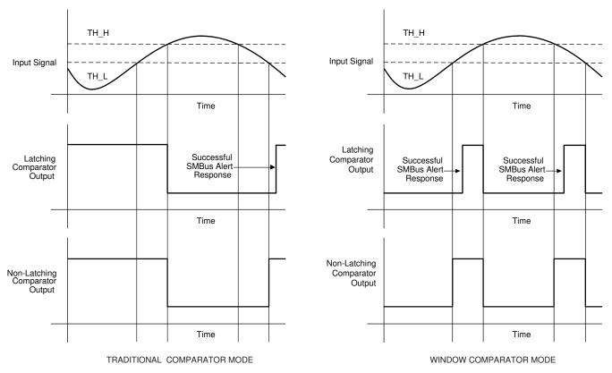
Figure 8-7. ALERT Pin Timing Diagram
