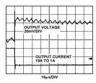
Figure 9. Transient Response, 19 A–1 A of Figure 2 Circuit
