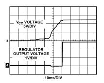
Figure 11. Power-On Start-Up Waveform
