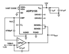
Figure 13. Closed-Loop Test Circuit for Accuracy
