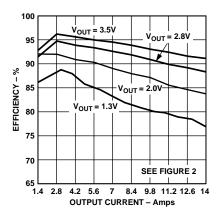
Figure 4. Efficiency vs. Output Current
