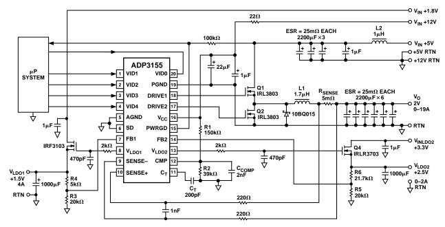
Figure 2. Typical VRM8.2/8.3/8.4 Compliant Core DC/DC Converter Circuit
