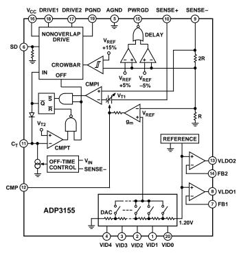
The ADP3155 contains two linear regulator controllers that are designed to drive external N-channel MOSFETs. These linear regulators are used to generate the auxiliary voltages (AGP, GTL, etc.) required in most motherboard designs, and have been designed to provide a high bandwidth load-transient response. A pair of external feedback resistors sets each linear regulator output voltage.
