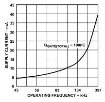
Figure 6. Supply Current vs. Operating Frequency
