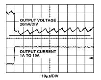
Figure 10. Transient Response, 1 A–19 A of Figure 2 Circuit
