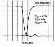
Figure 8. Driver Transition Waveforms
