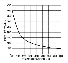
Figure 5. Frequency vs. Timing Capacitor
