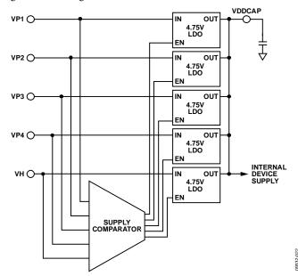
Figure 21.  $V_{DD}$  Arbitrator Operation
