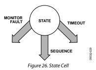
The ADM1166 offers up to 63 state definitions. The signals monitored to indicate the status of the input pins are the outputs of the SFDs.
