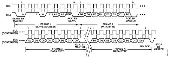
Figure 37. General SMBus Read Timing Diagram
