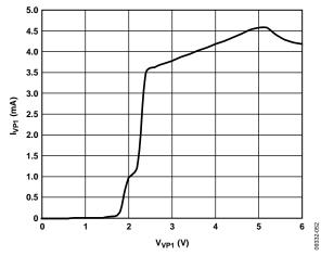
Figure 7. I<sub>VP1</sub> vs. V<sub>VP1</sub> (VP1 as Supply)
