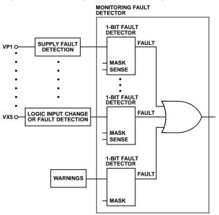
Figure 29. Monitoring Fault Detector Block Diagram
