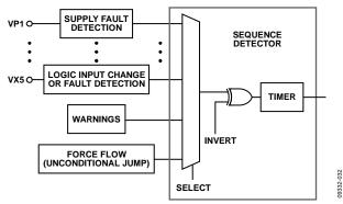
Figure 27. Sequence Detector Block Diagram
