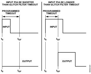
Figure 23. Input Glitch Filter Function
