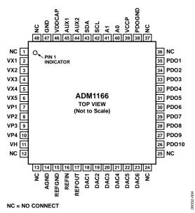
Figure 4. 48-Lead TQFP Pin Configuration
