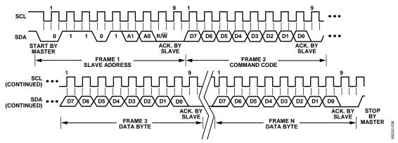
Figure 36. General SMBus Write Timing Diagram
