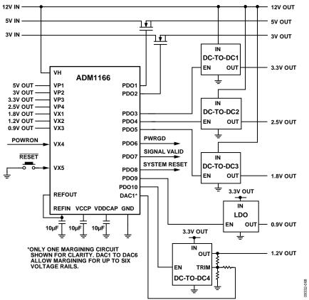
Figure 34. Applications Diagram
