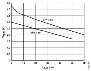
Figure 13. V<sub>PDO1</sub> (Weak Pull-Up to VPx) vs. I<sub>LOAD</sub>
