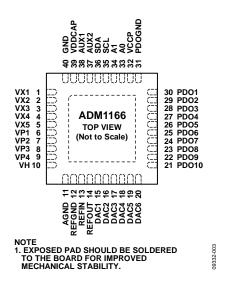
Figure 3. 40-Lead LFCSP Pin Configuration
