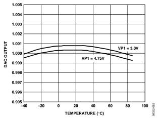
Figure 19. DAC Output vs. Temperature
