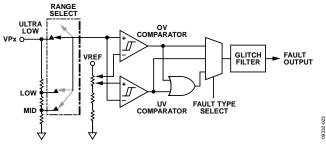
Figure 22. Supply Fault Detector Block
