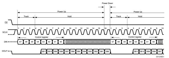
**ADC122S021 Operational Timing Diagram**
