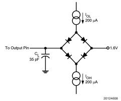
**Timing Test Circuit**
