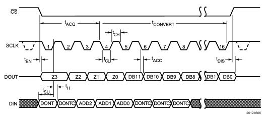
ADC122S021 Serial Timing Diagram
