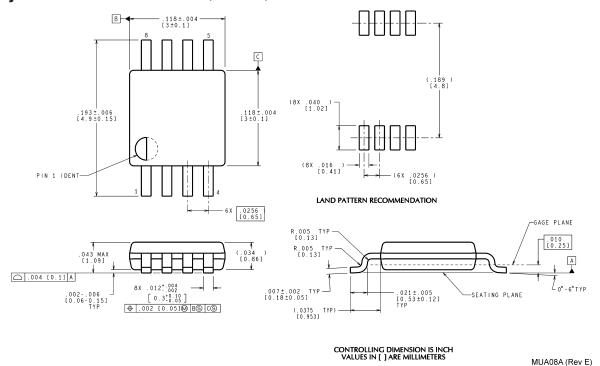
8-Lead MSOP Order Number ADC122S021CIMM, ADC122S021CIMMX **NS Package Number P0MUA08A**
