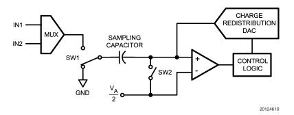
FIGURE 2. ADC122S021 in Hold Mode
