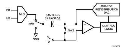
FIGURE 1. ADC122S021 in Track Mode
