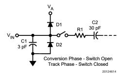
FIGURE 5. Equivalent Input Circuit
